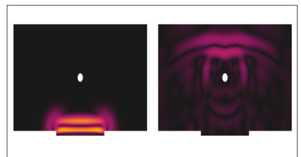
Displacement field at different time steps in a test block with a hole Own presentation
