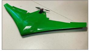
Green Raven GR001 Prototype, a 1:4 scale down of the MK18 kthaero.com/greenraven
