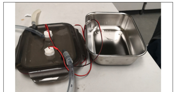
Lunchbox-Reactor with 2 UVC-LEDs installed. Own presentation
