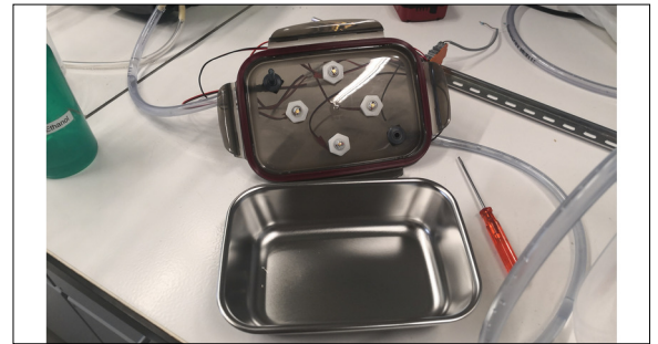
Lunchbox-Reactor with 4 UVC-LEDs in experiment setup. Own presentation
