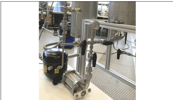
View on the built storage unit, with the compressor, the condenser (top right) and the mobile tank, which stores the DME
