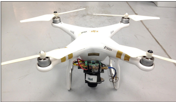
Drone equipped with infrared camera used in the aIRT measurements
