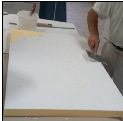
Figure 1: Preparation of XPS plate coated with the render.
