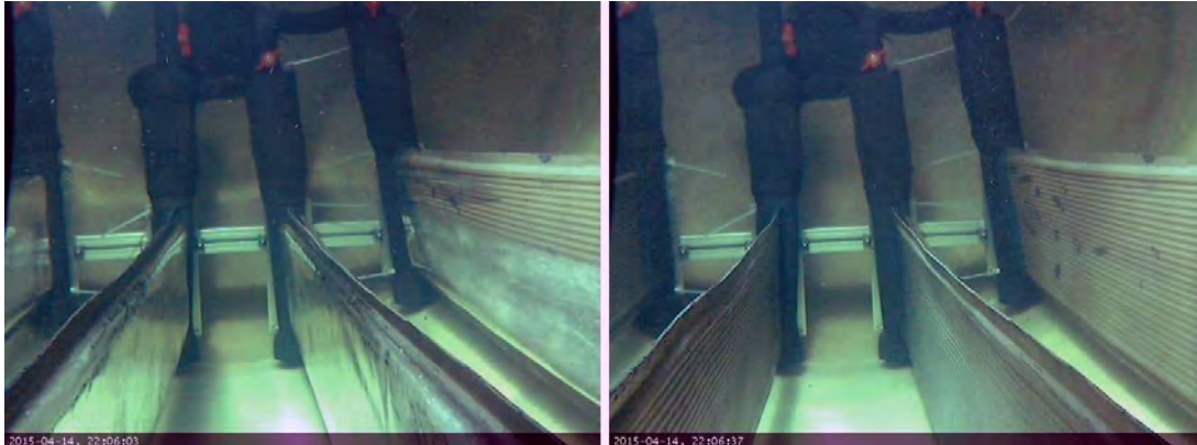
Figure 10.12: Four elastic heat exchangers with 1.6 m length each in the cylindrical ice storage before (left) and after (right) mechanical de-icing by inflating the heat exchangers.
