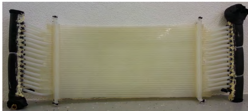
Figure 10.2: Flat heat exchanger plate made of silicone tubes that are cast in silicone
