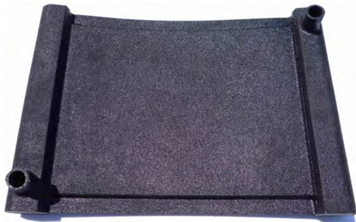
Figure 10.8: Functional model of the elastic heat exchanger printed in a 3D-printer.
