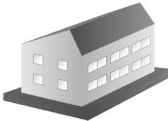
Figure 3.3: Schematic view of the building (showing south and west façades). The south roof is inclined 45 °. (Dott et al., 2012)
