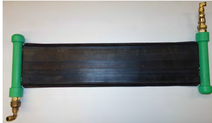
Figure 10.9: Heat exchanger with extruded EPDM plate for tests in the small ice storage.
