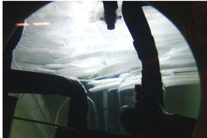
Figure 10.13: With de-icing detached and accumulated ice layers (white) that float in the cylindrical storage.
