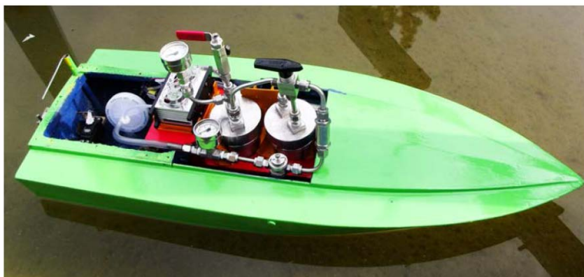
Figure 3: Model boat for the demonstration of hydrogen produced from aluminum in combination with a fuel for the propulsion of marine vessels by Gany et al. (2015).
