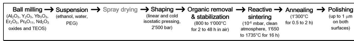
Figure 4: Manufacturing process for transparent laser ceramics.
