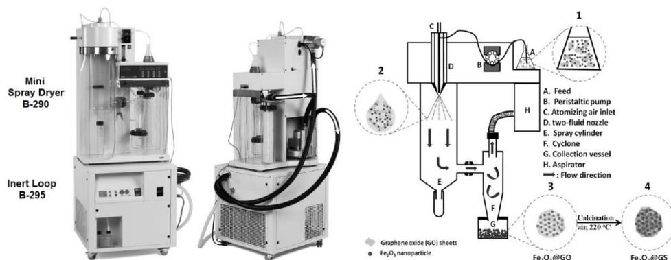
Figure 2: Mini Spray Dryer B-290 with Inert Loop B-295 (BUCHI Labortechnik AG) and schematic of spray drying of graphene-encapsulated Fe<sub>2</sub>O<sub>3</sub> nanoparticles (Fe<sub>2</sub>O<sub>3</sub>@GS) [3].
