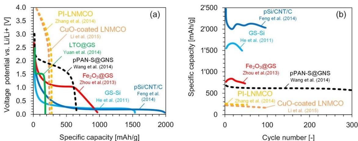
Figure 3: Voltage profiles (a) and cycle performances (b) of spray dried anode materials (solid lines, LTO@GS [1], Fe<sub>2</sub>O<sub>3</sub>@GS [3], GS-Si [6], pSi/CNT/C [12]) and cathode materials (dashed lines, PI-LNMCO [14], CuO-coated LNMCO [15], pPAN-S@GNS [2]).
