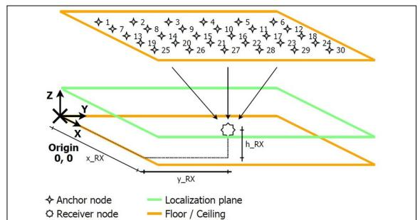
RSSI input samples of the training data set sorted according to the receiver position on the localization area.
