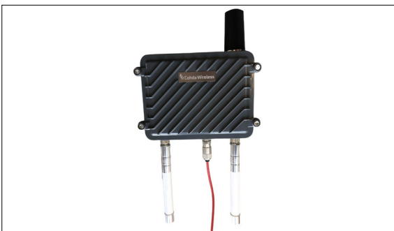
The Roadside unit with a GNSS antenna and two V2X antennas Own presentment
