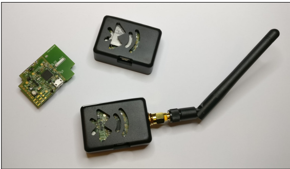
Top: low-power device with integrated battery and chip antenna. Bottom: relay device with external antenna
