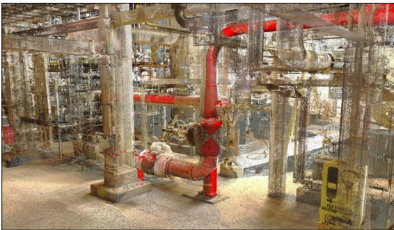
3D-model: It consists of distance data as a point cloud which has been colorized according to the color images. Source: kleinfelder.com 3D Reality Capture Solutions
