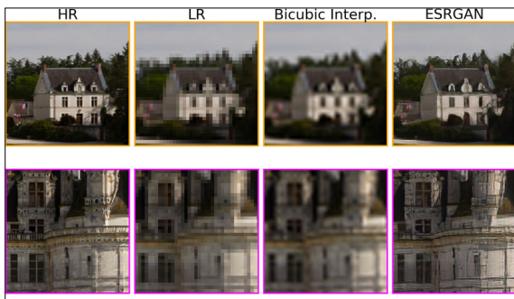
Comparison image versions: ESRGAN-image (right) is almost indistinguishable from HR-image (left). [4x upscaling] Own presentment
