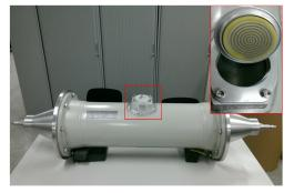
Figure 1, GIS dummy for sensor measurements
