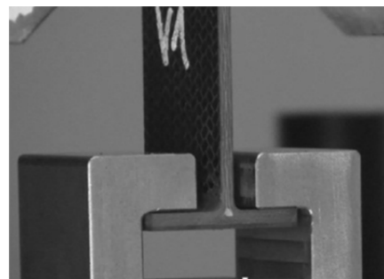
Figure 5: U-channel (left) and T-section (right) in testing machine
