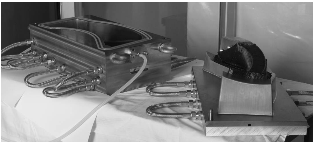
Figure 5: RTM tool (left: lower die; right: upper die with preform and core)
