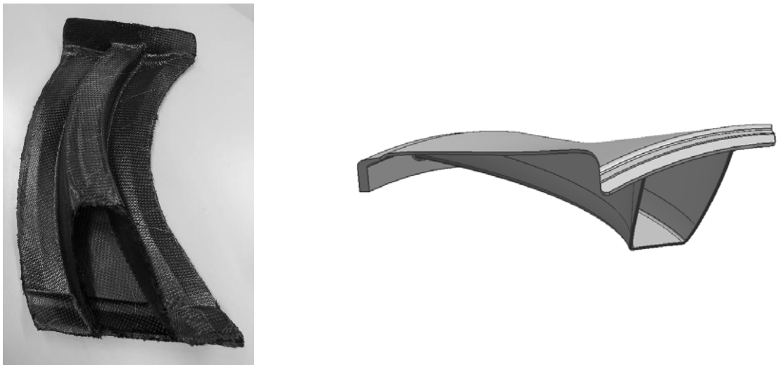
Figure 3: Preform and moulded shape of filler
