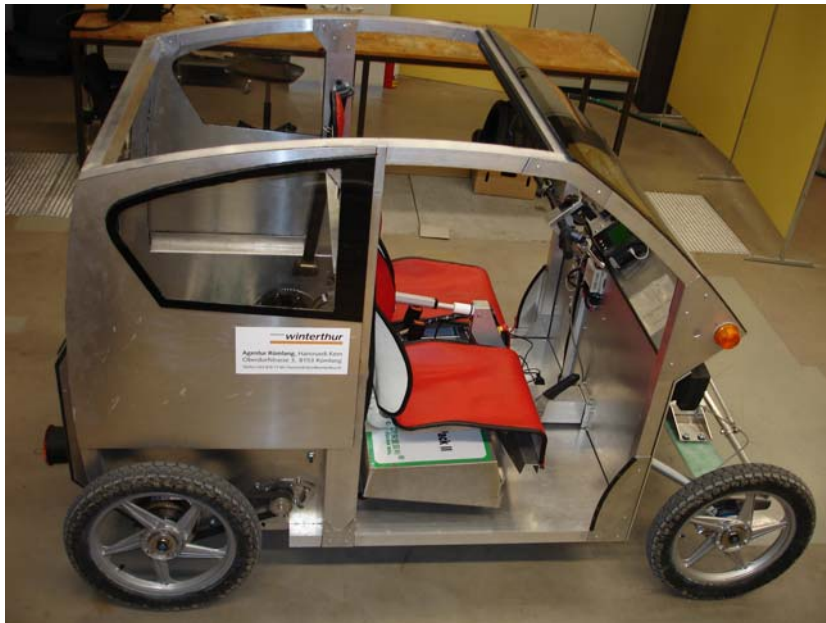
Figure 5: The pre-prototype, without front-end, doors or inside finish
