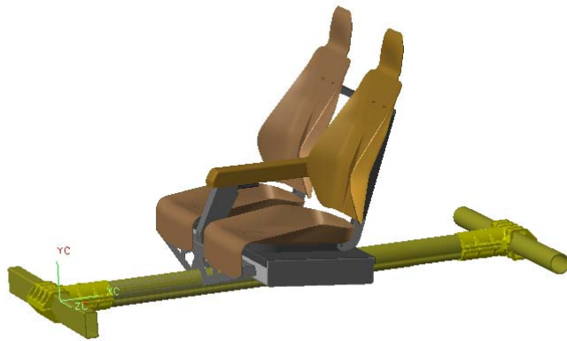
Figure 2: The longitudinal torsion beam with the rigid axles and the spring-mounted seats
