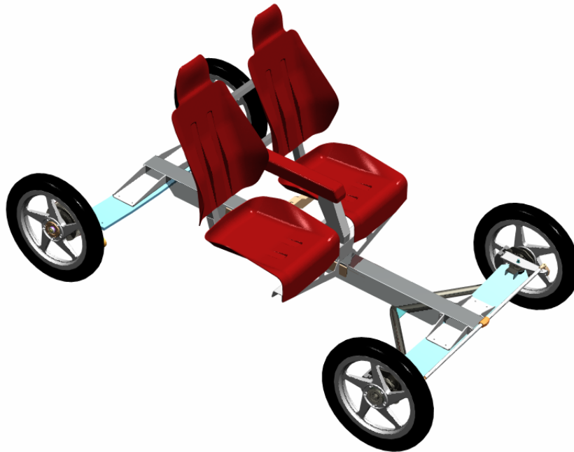
Figure 6: Reworked chassis with leaf springs and special tyres
