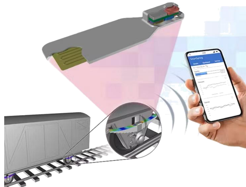
CSEM Long-term heavy-duty springs monitoring sensor
