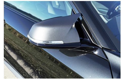
SLS 3D printed final product in PA12 and painted
