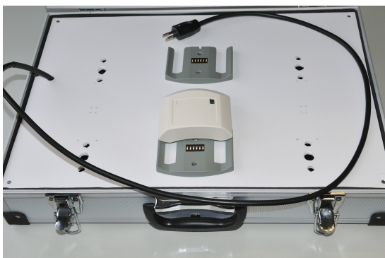
Charging case with 2 of 6 fully mounted charger stations. Tag half way inserted into charging station.
