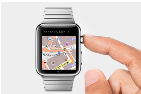
Map of the current location. By using the digital watch crown one can zoom in and out.
