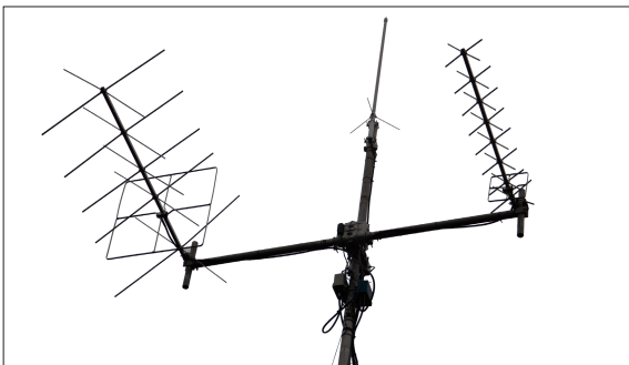
HSR ground station antenna mast with two x-quad and one multiband monopole antenna
