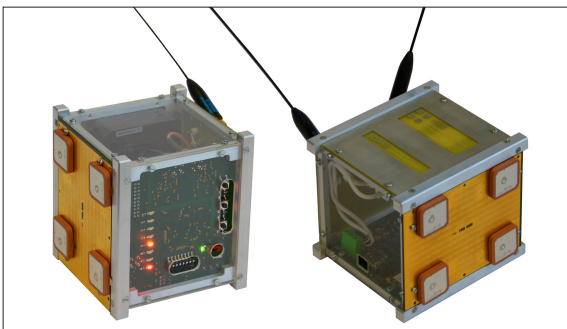
Developed HSR DemoSat with receive, transmit and GPS antenna
