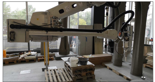
Figure 1: Concrete 3D printer at the ETH Zürich with printed structures in the background Own presentation
