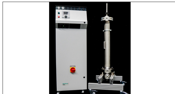
Temperature control system by Regloplas (left) for the operation of the SEM reactor manufactured by Fluitec (right). Samuel Hecht, UMTEC/OST
