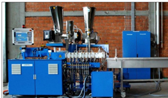
Compoundieranlage IWK, ZSK 26
