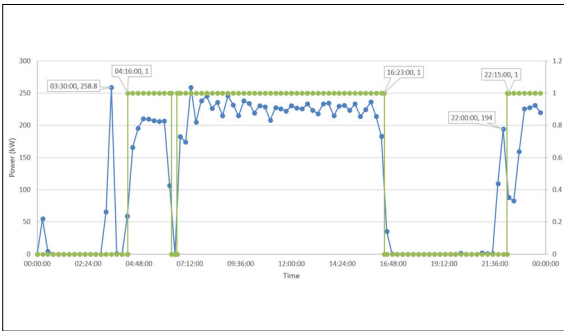
Graph that depicts the power consumption and the presence of a product (secondary axis) vs the time (1-day period)
