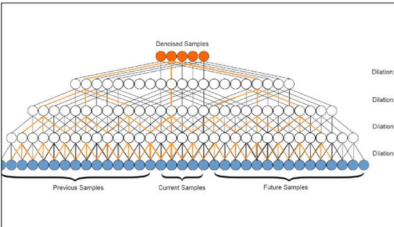
The dilated convolutions in the modified Wavenet. The Non-causal structure predicts a target field from input samples. D. Rethage, A wavenet for speech denoising
