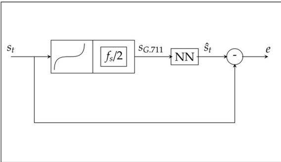
The task of the neural network is to minimize the error  $e$ , based on the signal received by a phone call. Ozhiker, Graph of -law a-law algorithms,
