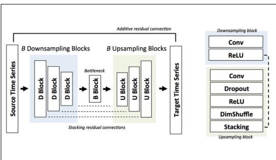
Deep Residual Neural Network of the Super Resolution network. On the right, sublayers of the down and upsampling layers. V. Kuleshov, Audio super resolution using neural networks
