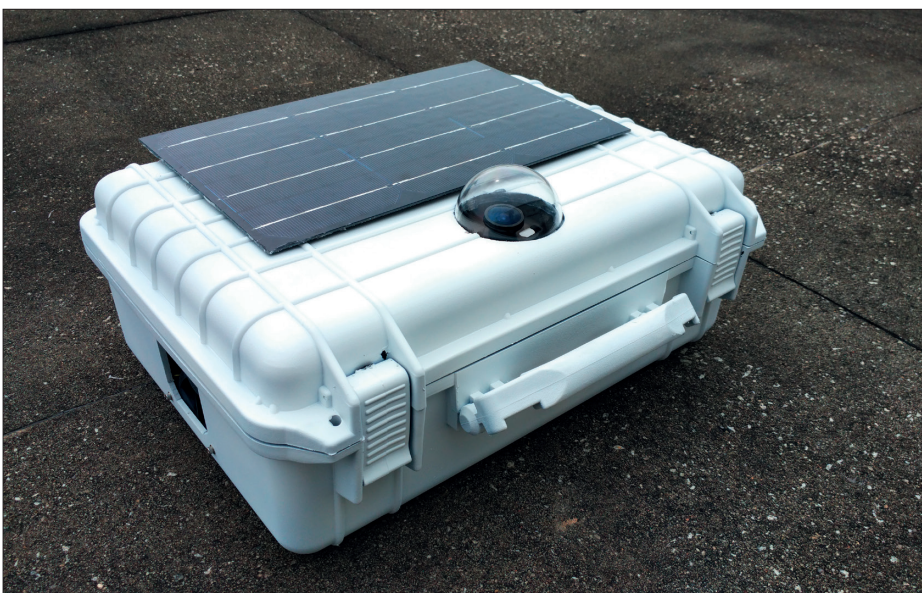
Prototype Housing with Solar Module
