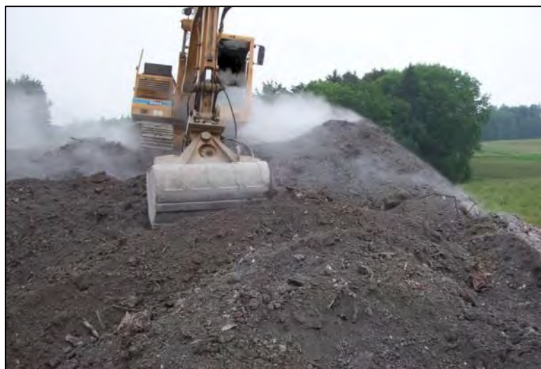
Fig. 1.1: Bottom ash from a Municipal Waste Incinerator before processing. Exothermic chemical reactions cause to a marked increase in temperature which results in the evaporation of a significant amount of moisture.
