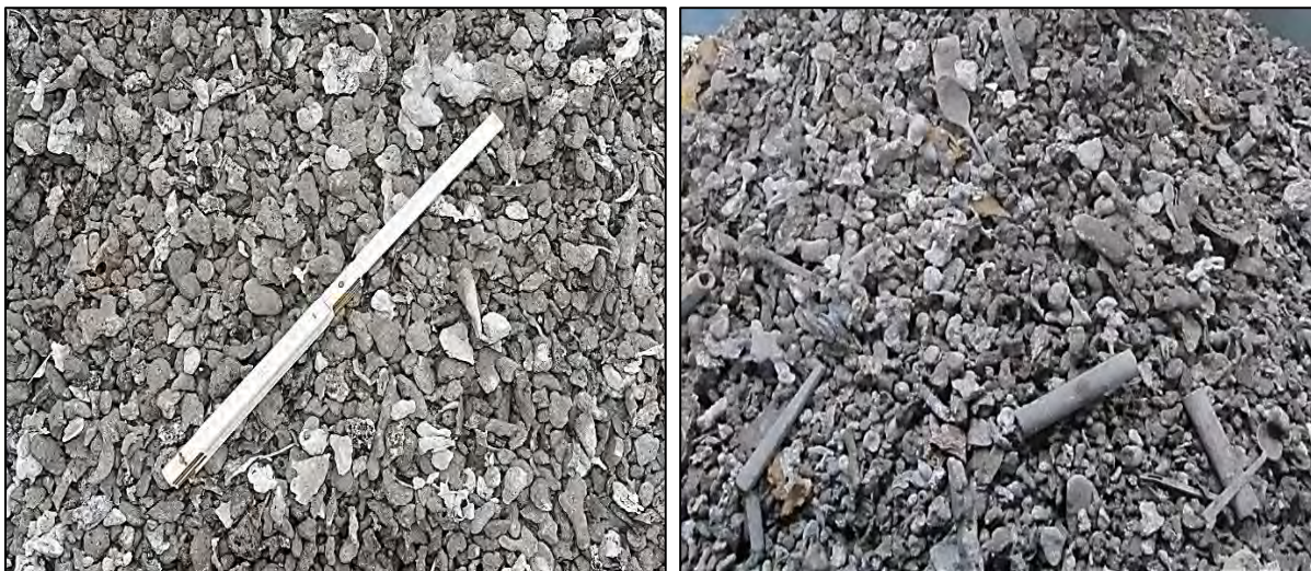
Fig. 4.21: Coarse NF recovered by ECS: (left) mostly aluminum. (right) NF concentrate from a sensor sorter (after ECS): mostly SS including substantial amounts of silverware.
