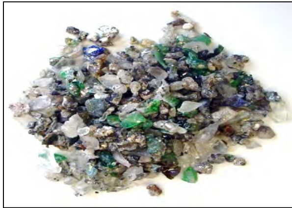
Fig. 2.9: Glass in BA: 4-8 mm
