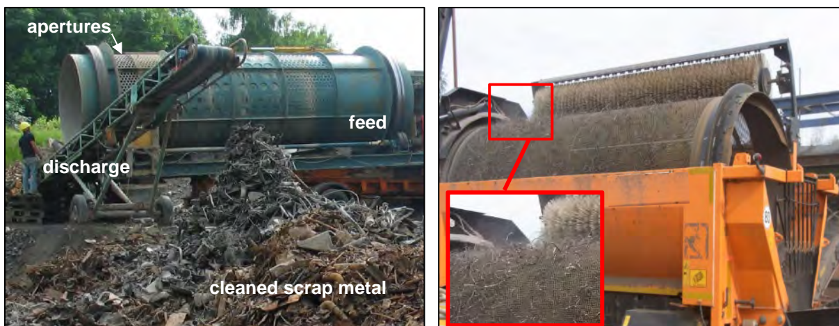
Fig. 4.7: Coarse classification of BA on trommel screens.
