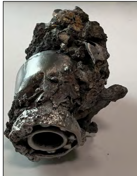
Fig. 2.11: (left) Slag particles with locked pieces of metals and ceramics. (right) Metal objects (e.g. a ball bearing) being encapsulated by a slag matrix.
