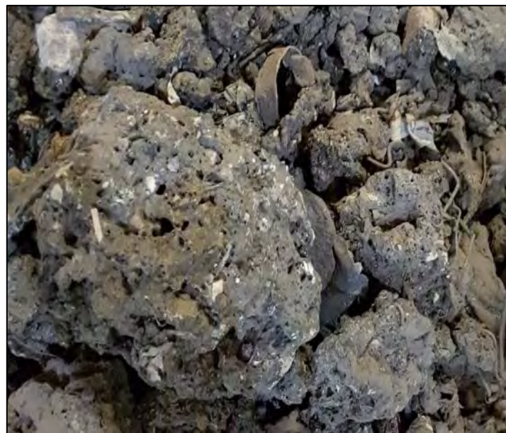
Fig. 2.11: (left) Slag particles with locked pieces of metals and ceramics. (right) Metal objects (e.g. a ball bearing) being encapsulated by a slag matrix.
