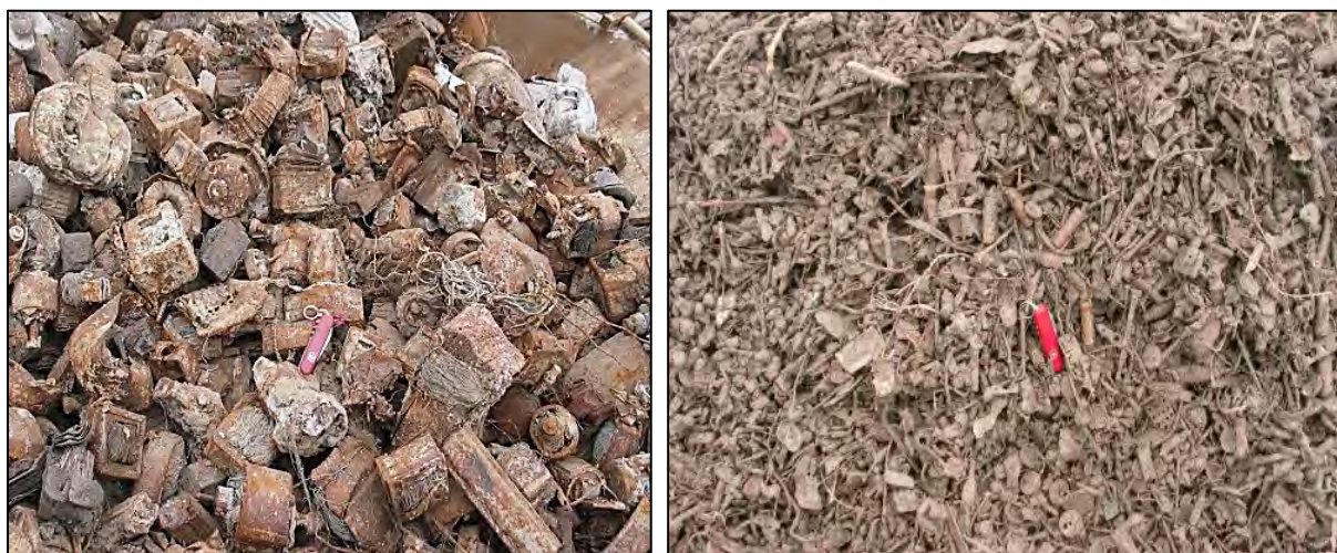
Fig. 4.24: (left) Transformers and electric motors handpicked from BA.(right) Despite the separate collection of batteries in Switzerland the magnetic concentrate 8-32 mm contains some 1-2% batteries. As steel mills are not equipped with adequate flue gas treatment, the batteries should be manually removed for environmental reasons but this is not usually done due to excessive cost.
