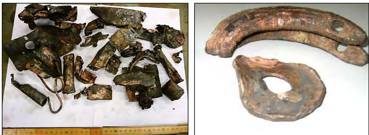
Fig. 3.8: Copper plated pieces of steel recovered from BA (after removal of the oxide scales by shredding).
