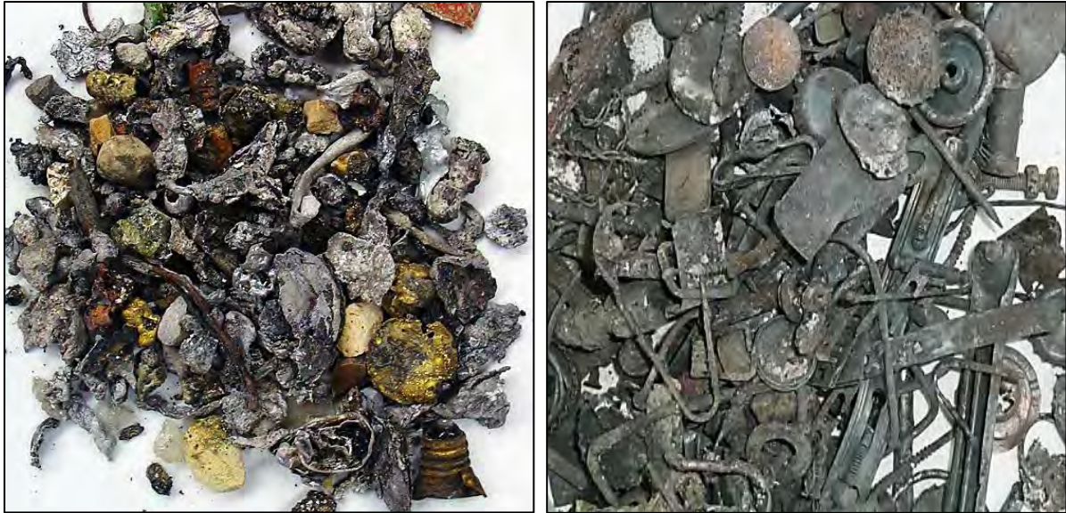
Fig. 5.4: Metals 10-40 mm recovered from dry extracted BA: NF (left) and FE (right). Even thin foils of aluminum have been successfully recovered as a pure product with virtually no corrosion and adhesions of mineral material.
