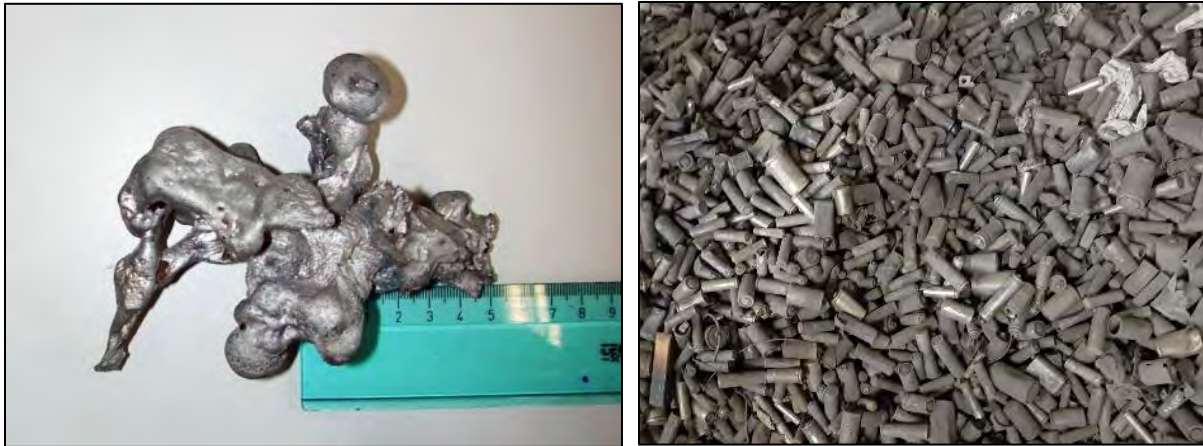
Fig. 3.3: Aluminum melt solidified as “nugget”.
