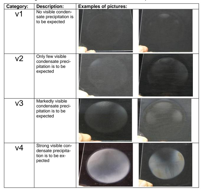
Table 2: Change of transmittance on the condensation traps
