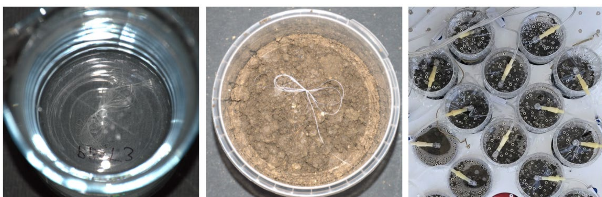
Fig. 3: Biodegradation experiment, close up: in filtered freshwater from a natural pond (left), on soil from a backyard (middle) and the sample in the soil with an irrigation system (right).
